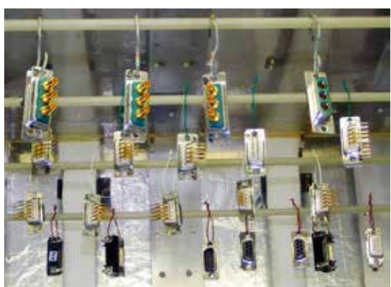
Storage of the test object during the mixed gas exposure
